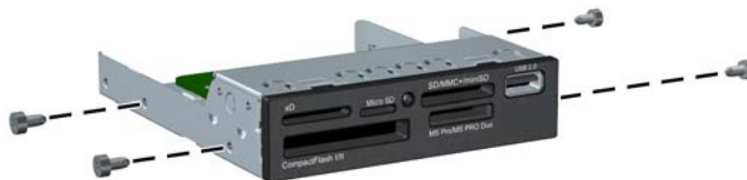
Figure 4-30 Installing Guide Screws (Media Card Reader Shown)
